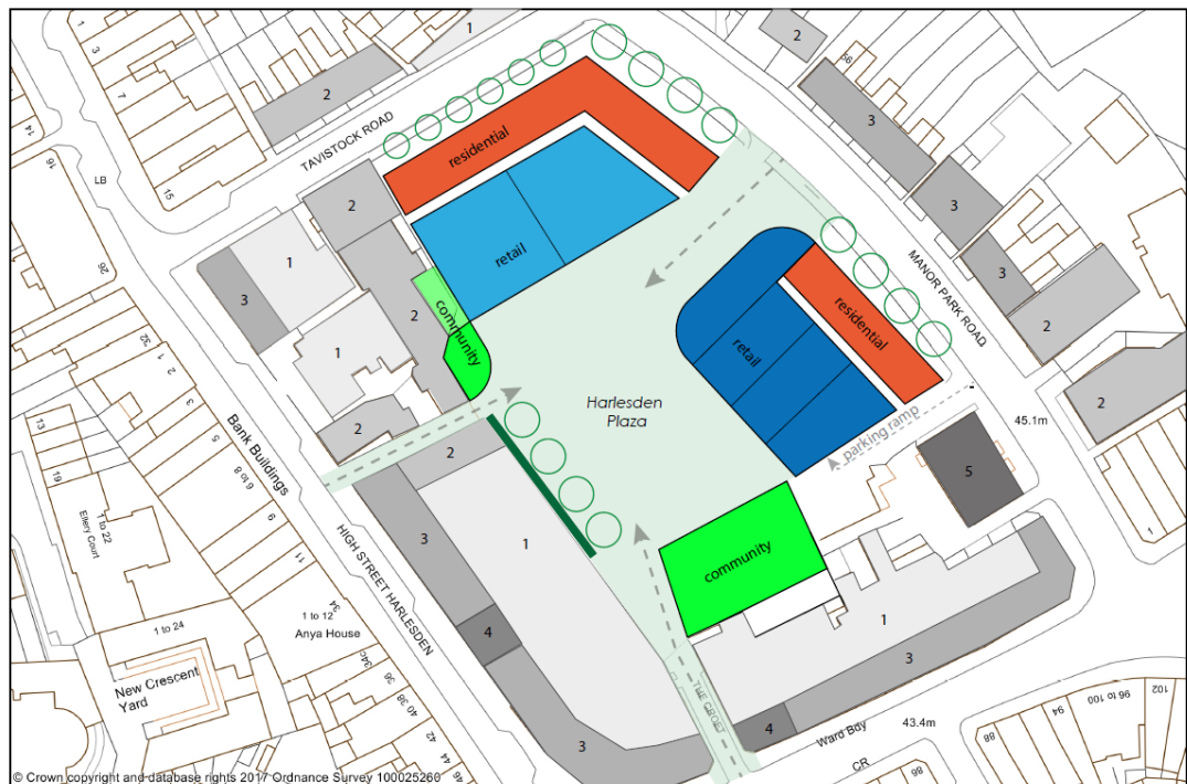
Fig.21 below, Example diagram of how Harlesden town square could be laid out, including proposed ground-floor uses
